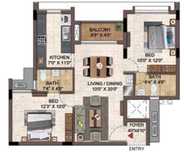
UNIT NO - A G01 - A 401, A G02 - A 402 A G03 - A 403, A G04 - A 404 D G01 - D 401, D G02 - D 402 D 103 - D 403 TYPICAL FLOOR
